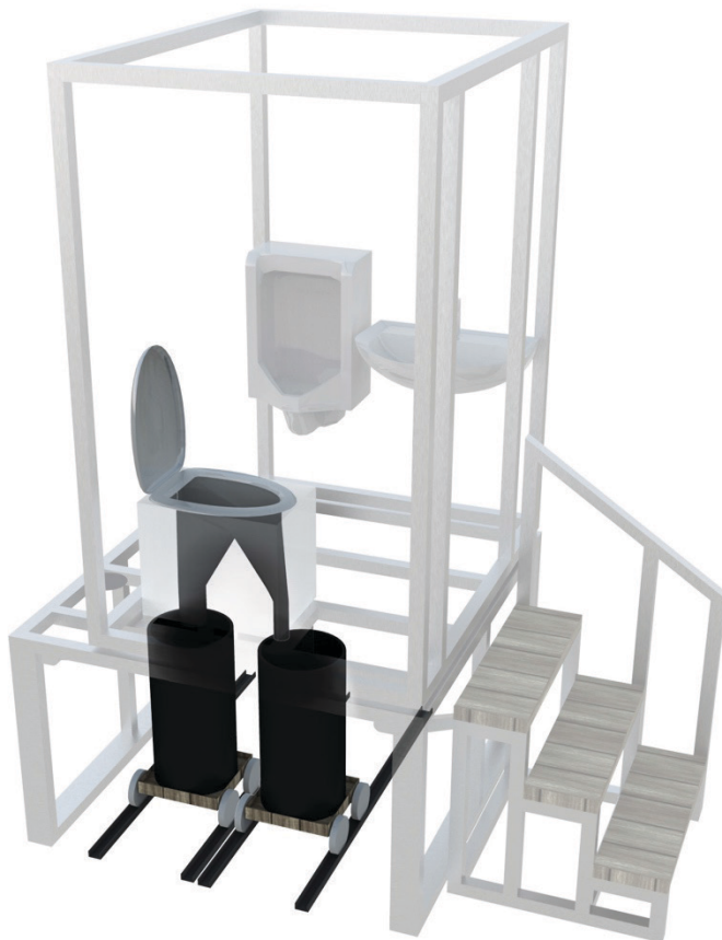
Figure 30: Draft design of iPiT® with main parts of user interface: toilet seat and collection bins (based on ACF Mongolia)
